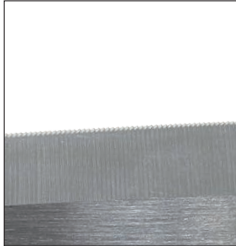
Nano-serrations (Serration pitch 0.3mm)
