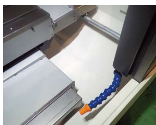
Coolant unit with chip flush (spot gun provided)
