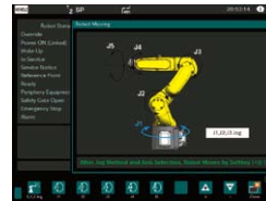
Robot manual operation screen
