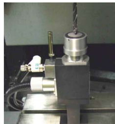
Tool length switch for automatic measurement
