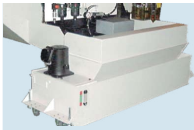
Coolant unit (tank)
