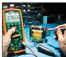
Measure the insulation resistance of transformer windings
