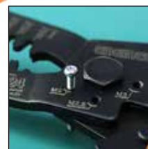
Screw Cutter M2, M2.6, M3 (Min. Thread Length: 3.5mm)
