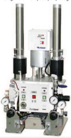
The EP1320C tandem cartridge pump is designed to easily transfer material for controlled dispensing via a high pressure valve. The suitable viscosity range is 10,000cps - 600,000cps. Rated at 15:1 the system provides a maximum of 995 psi regulated material pressure. The A & B cartridge management automatically switches from either A to B or B to A when the cartridge is exhausted. Cartridges are contained in metal jacketed cylinders.
