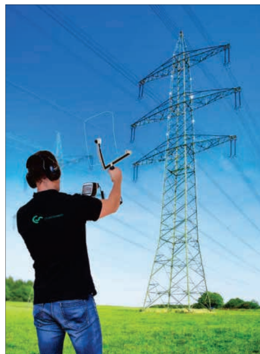
Checking high voltage overhead lines for corona discharge
