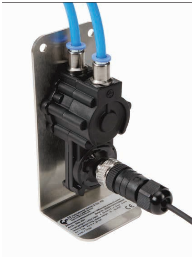
Typical operation of the differential pressure sensor: Connection with two PE hoses before and after the filter element.
