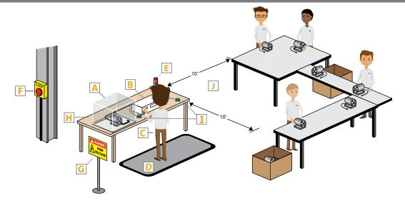
One of the best ways to prevent injury is to ensure that your test station is set up safely and securely. Test stations can be setup with or without direct protection depending on your requirements. Direct protection means that the operator cannot physically come into contact with an energized DUT while a test is running. This safe workstation diagram uses a Hipot tester as an example to illustrate how our protective equipment can be used to keep operators safe.
