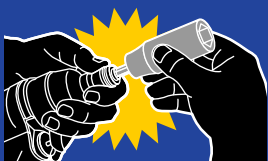
The shaft is retained to match tool angle, so the socket fits the ball.
